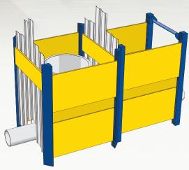
Linear Tight Shoring System utilizing in line Utility Crossing Frame
